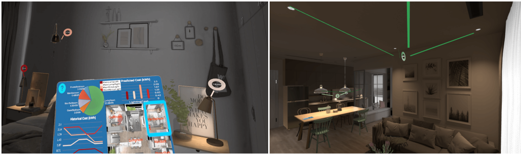
Fig. 1. Images of our prototype for situated analytics using hybrid user interfaces, simulating AR in VR. Left: In the foreground, the user holds a tablet at chest height with a dashboard of situated visualizations that show energy usage data of lights in the apartment. In the background, embedded visualizations of energy usage are next to their respective lights. Right: The apartment's living room and kitchen with more embedded visualizations. Leader lines connect each embedded visualization to one or more lights that it relates to.
