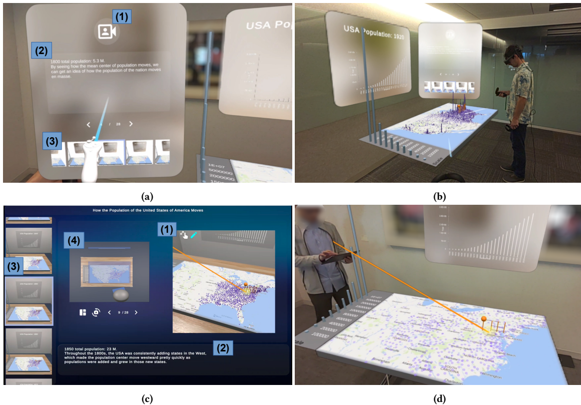
Figure 2: Screenshots from our augmented presentation system in use. (a) Symmetric presenter interface (close-up view). Features: (1) Button to toggle a mirrored view showing a simulated view from the audience’s perspective. When activated, the simulated mirrored audience view appears directly above the pictured interface. (2) Speaker notes to guide the presenter on the presentation. (3) Scene switcher with a carousel view of previews of each scene in the presentation. (b) “Zoomed out” presenter’s view of the presenter interface, the presentation content, and the audience. (c) Asymmetric presenter interface for the tablet. Features: (1) Simulated mirrored audience view. The presenter can tap on the virtual content to cast a virtual pointer ray. The presenter can press the hand icon button to switch to map interaction mode, allowing them to zoom the map by pinching with two fingers or pan the map by moving one finger. (2) Speaker notes. (3) Scene switcher. (4) Top-down view with simulated audience head to visualize the audience’s position and orientation relative to the presentation content. The presenter can tap the presentation surfaces shown in this view (the map and the slide behind the map) to stabilize the simulated camera view so that it focuses on these objects. (d) Audience’s perspective of the presenter using the virtual pointing ray when using the asymmetric presentation modality.
